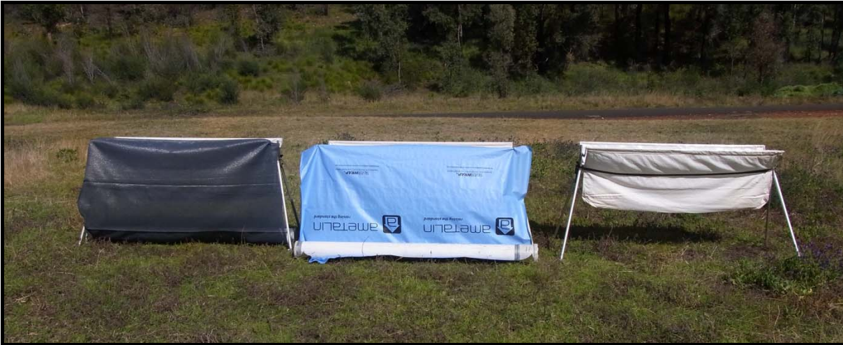
Figure 1. View from the eastern side of the three trap bag assemblies with, from left to right, shade cloth, sarking and no shading.
