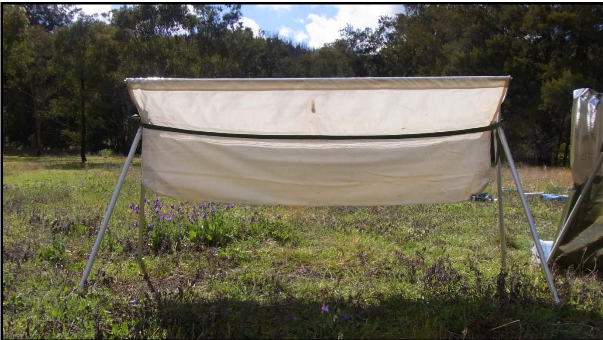
Figure 2. The view in mid-morning from the western side showing the silhouette of a temperature sensor placed between the internal plastic lining and the cloth outer shell of the trap bag.
