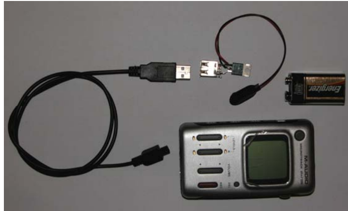
Figure 2. The Microtrack takes a mini USB connection, and the remainder connects in the sequence shown.
