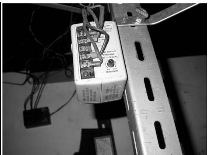
Figure 3. The IR door beam (12 V power and relay connectors).
